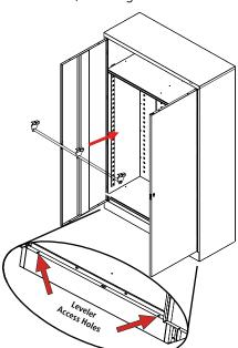
on the far right and far left side. The open side of the side brackets should face into the unit. Place the last bracket on the coat rod (Ref. No. 10) and insert the rod into the other by flexing the second bracket. Secure the bracket to the middle of the shelf with one bolt and nut through the hole provided in the center of the shelf. At this time, tighten all of the nuts and bolts around the entire unit.
