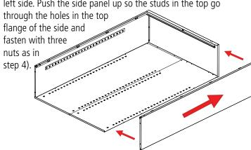
**6.** Attach the sill (Ref. No. 8) to the sides. Place nuts loosely on each of the studs and slide the ends of the sill into the slots on both sides of the unit. Then, securely tighten the nuts.
