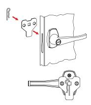
With the handle still in the open position, hook the locking bars (Ref. No. 11) to the locking cam (see "A" at left). Once in position, slowly rotate the door handle to the closed position so the lock bars prot rude from the holes at the top and bottom of the door (shown at right, below).
